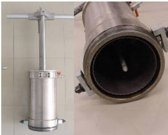
Figure 3 : The specialized hot tapping tool
